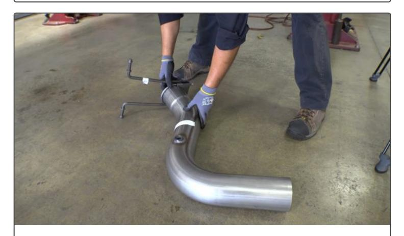
7. Install a 5" exhaust clamp onto the inlet of the Rear Tailpipe & Install the Rear Tailpipe onto the outlet of the Front Tailpipe.
